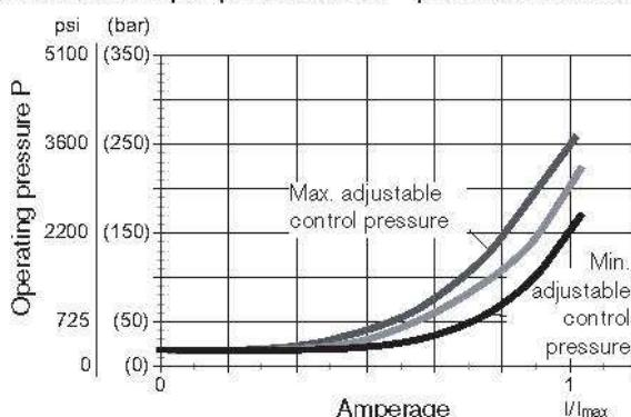
Hysteresis static current-pressure characteristic < 45 psi (3 bar)
