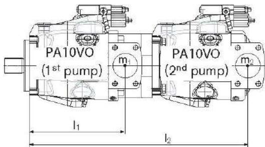
m<sub>1</sub>, m<sub>2</sub>, m<sub>3</sub> Mass of pumps [lbs (kg)]
