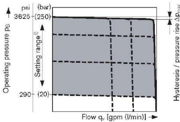
**i)** In order to prevent damage to the pump and the system, this setting range is the permissible setting range and it is not allowed to be exceeded.
