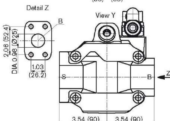
Dimensions of service line ports turned through 180° for counter-clockwise rotation
