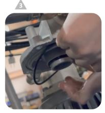
再將其放入濾心座內部的油封溝槽中。 Place it into the inner seal groove of the filter base.
