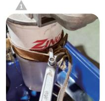
將罐體<mark>順時針</mark>旋轉鬆開後,更換新品。 Loosen the canister by turning it <mark>clockwise</mark>,
